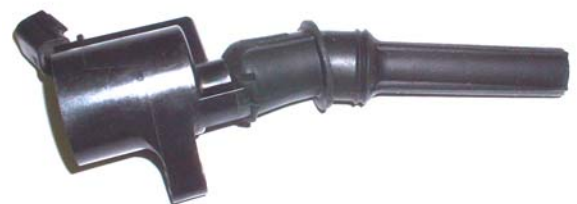
5 – Finished assembly. The use of silicone di-electric grease is highly recommended inside the bottom of the COP boot. This will ease later removal and help keep moisture and damaging contaminants out of the boot.
