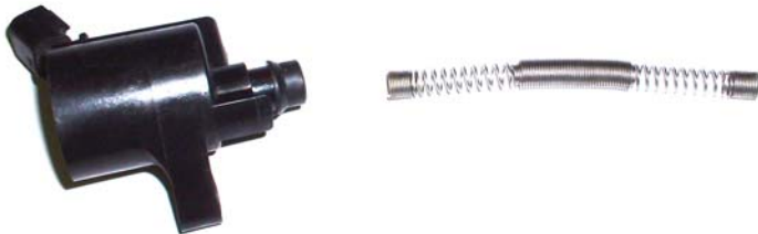
2 – Remove the old spring conductor from the coil, clockwise rotation of the spring while gently pulling will simplify removal. Some COP boots have the spring as an integral part of the boot and this step will not be necessary.
