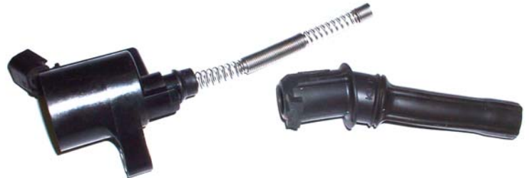
1- Remove the COP boot by firmly pulling away from the coil.
